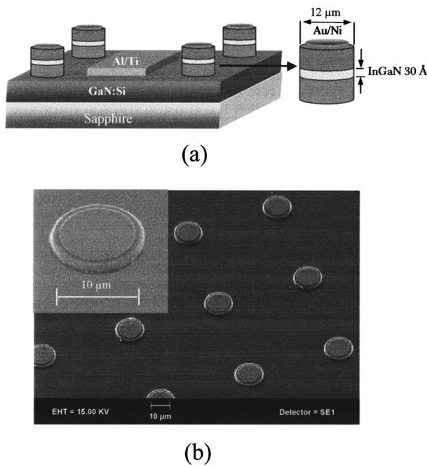
FIG. 1. (a) Schematic diagram and (b) SEM image of InGaN/GaN QW microsize LEDs ( $\mu$ -LEDs).
