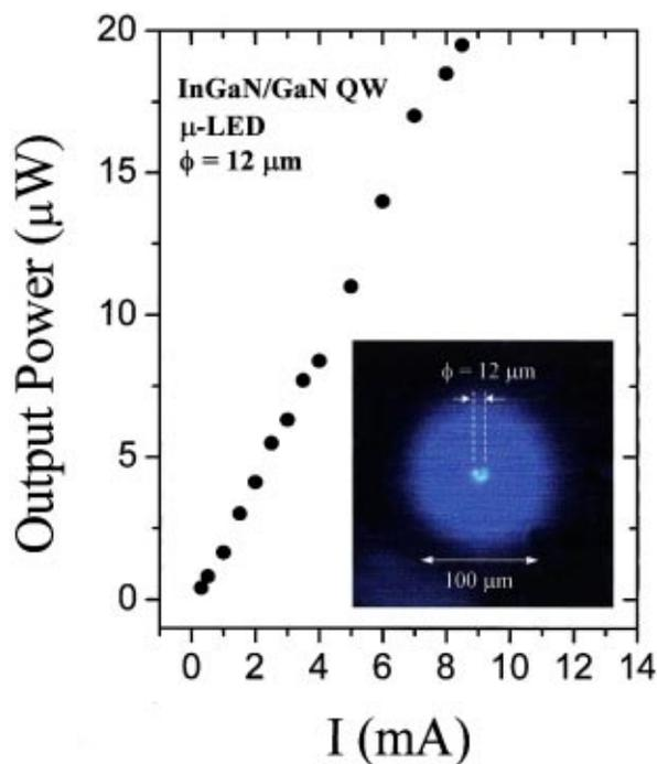
FIG. 4. (Color) The total output power as a function of forward current ( $L$ - $I$  curve) for one of our unpackaged InGaN/GaN QW  $\mu$ -LED measured in the sapphire substrate side. The inset is an optical microscope image taken from the top of the  $\mu$ -LED. The bright spot of 12  $\mu\text{m}$  in diameter in the center is the area of  $\mu$ -LED operating at a forward current of about 5 mA.
