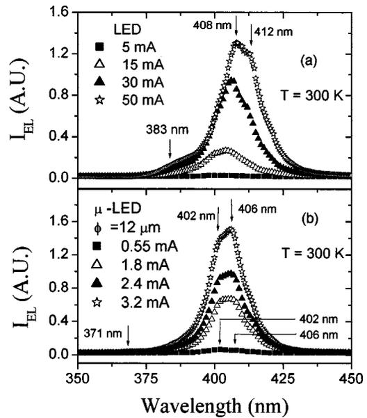
FIG. 3. 300 K electroluminescence (EL) spectra of an unpackaged (a) InGaN/GaN QW conventional broad-area LED and (b)  $\mu$ -LED measured under dc biased conditions for several different forward currents.
